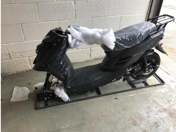
Carefully remove the cardboard packaging and unwrap all of the parts from their protective covering. When cutting the adhesive tape take care not to damage paintwork. Identify the parts and ensure that none of the smaller items are discarded with the packing.
