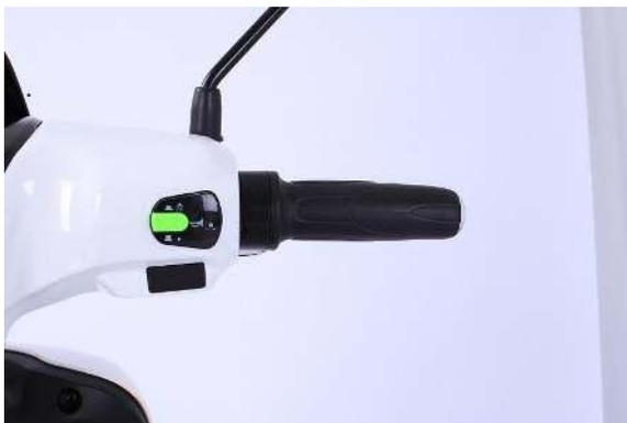
The throttle is operated by the right handle on the handlebar which also has the on/off switch for the lights and a horn.
