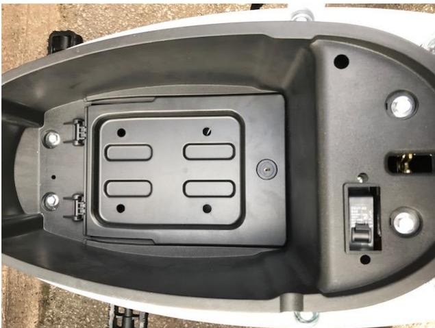
Turn the grey trip switch to the **off** position then unlock the battery panel with the ignition key and lift it up. Unplug the battery and remove it with the strap.
