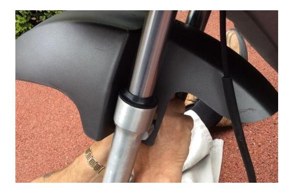
Take the front wheel and ease the brake mechanism into the drum.
