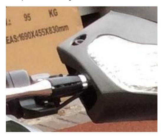
Having pressed the mirror bolts fully home, tighten the securing nut with a spanner. Before fully tightening, adjust the mirror angle to suit your riding position.
